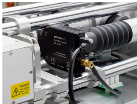
Real time beam profile monitoring option
