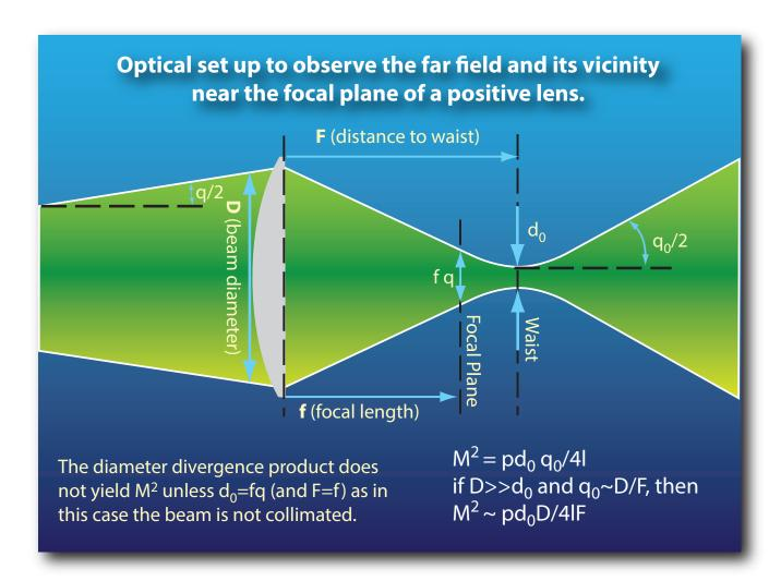
**A** true measure of the quality of a laser beam is the parameter known as M<sup>2</sup>, also referred to as a number of 'times diffraction limited'. It describes how a beam will diverge compared to a theoretically 'perfect' laser beam of the same wavelength and initial size that has the lowest possible divergence given by diffraction theory. A theoretically perfect laser beam must have a Gaussian intensity distribution whereas most real laser beams do
