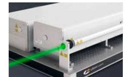
LPY7000 with additional 10J output stage doubled to 532nm outputting 5J at 1Hz, beam diameter 25mm.
